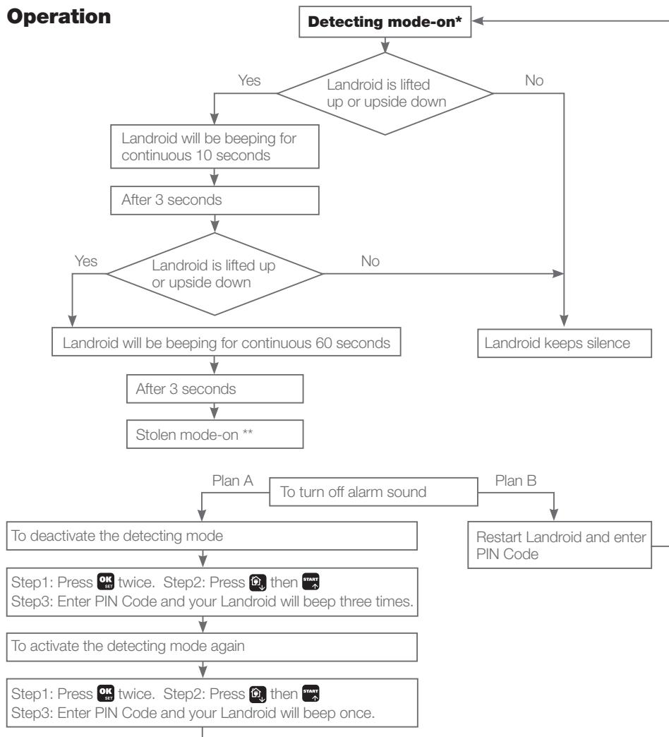
\*Detecting mode-on: The alarm function will be enabled. Moreover, thanks to the battery in the module, your Landroid also can support this function when it is power-off.
