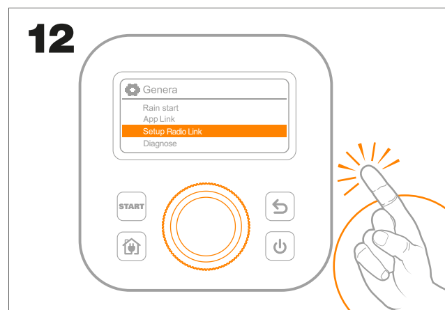
12. Rotate the knob to select the menu item "Setup RadioLink", then press the knob to confirm
