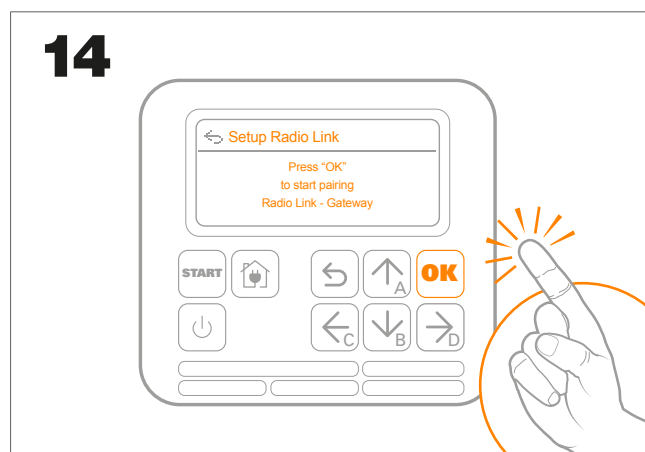
14. The wording “Press OK to start pairing RadioLink – Gateway” will appear, press OK
